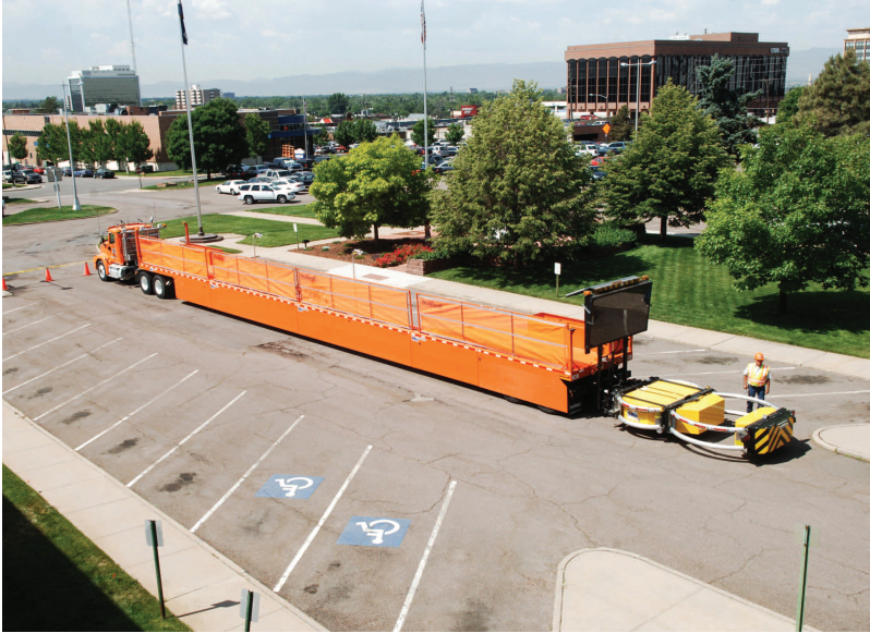
Photo 3: The mobile barrier trailer (MBT-1) is a rigid-wall trailer that serves as a structural and visual barrier between a highway construction worksite and active roadways.
